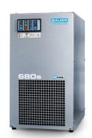
The refrigerant type dryer B-KOOL by BAUER cools the compressed air and extends the filter cartridge life time. The B-KOOL unit is integrated into the high pressure piping of the compressor after the final oil and water separator. It can be mounted on top of an unit with Super Silent housing or placed separately.
